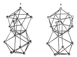
Figure 2. Condensed units of boron icosahedra and icosahedral fragments: a,  $B_{20}$ -( $C_2$ ) unit, found in  $\alpha$ -AlB<sub>12</sub> and  $\gamma$ -AlB<sub>12</sub>; b,  $B_{20}$ -( $C_s$ ) unit, found in  $\gamma$ -AlB<sub>12</sub>.
